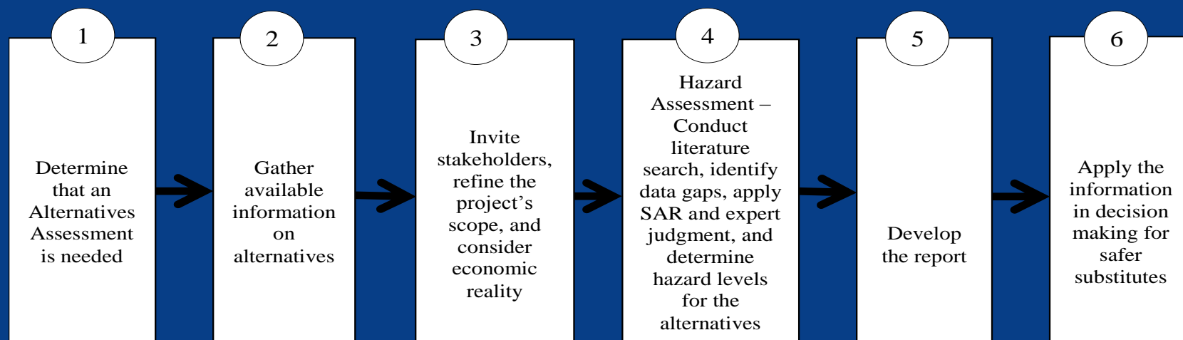
Six Broad Steps in Conducting a DfE Alternatives Assessment (From Lavoie et al. 2010)
